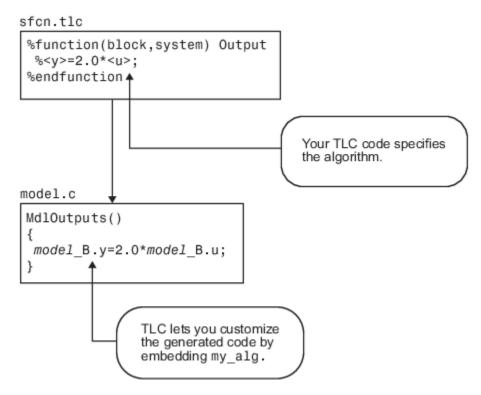
The S-function timestwo.c provides a simple example of a fully inlined S-function. This block multiplies its input by 2 and outputs it. The C MEX version of the block is in the file <code>matlabroot/toolbox/simulink/simdemos/simfeatures/src/timestwo.c</code>, and the inlining TLC file for the block is <code>matlabroot/toolbox/simulink/simdemos/simfeatures/tlc c/timestwo.tlc</code>.
