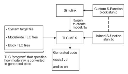
A TLC program is a collection of ASCII files called scripts. Because TLC is an interpreted language, there are no object files. The single target file that calls (with the %include directive) other target files used for the program is called the entry point.
